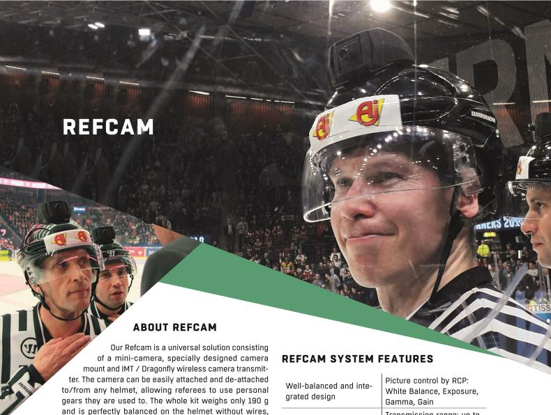
Refcam can be mounted on most helmets, including those used in hockey, horseracing, and football. This POV system also bears the possibilities of being arranged as a wearable chest- or ear- cam solution. Battery charge can last up to several hours and the battery compartments allow easy replacement of the battery during the game breaks. During the operations, the camera is remotely controlled by RCP placed in the OB-VAN that comes along with the kit.
