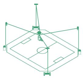
3D mode: four power winches are used to move the dolly within 3D space between the pulleys.
