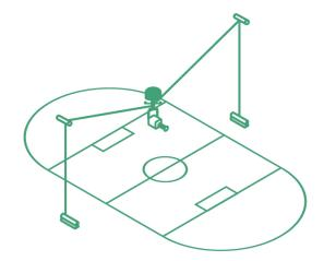
2D mode: two power winches form a working zone as a vertical plane between the pulleys.
